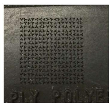
The sample in the image was subject to rapid aging tests that simulated a desert environment and was still decodable even though the sidewall exhibited significant cracking.
